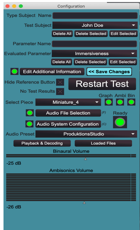
Fig. 5, Configuration window for the MUSHRA test. Here the name of the evaluated room parameter, the name of the tester, the selection and loading of the test signal and the calibration of the amplitude ratio between the binaural and the ambisonic test file can be set.
