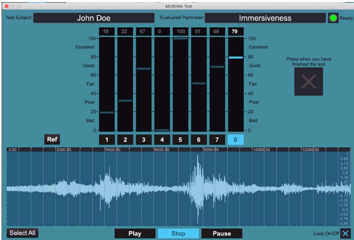
Fig. 4, User interface to the test program of the MUSHRA test.
